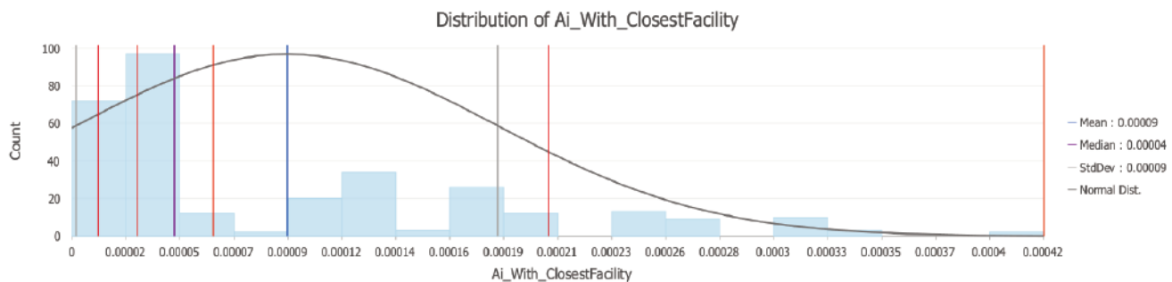
Figure 7. The 1,500-meter accessibility score histogram based on 2SFCA. Districts with a 0 scores were excluded from the results. The vertical, red lines are the classification breaks.
