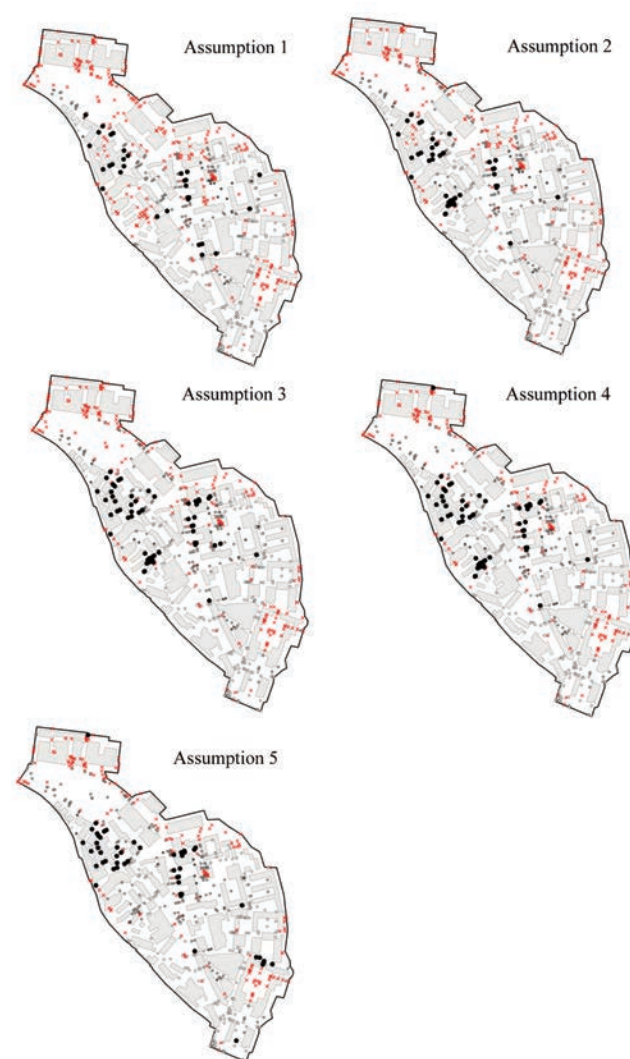
Figure 6 Wheelchair cold spots in the KTH campus. The crosshairs (in red) indicate completely inaccessible nodes, while the dots (in black) indicate substantially less accessible nodes. Each map corresponds to one of the six wheelchair mobility assumptions.
