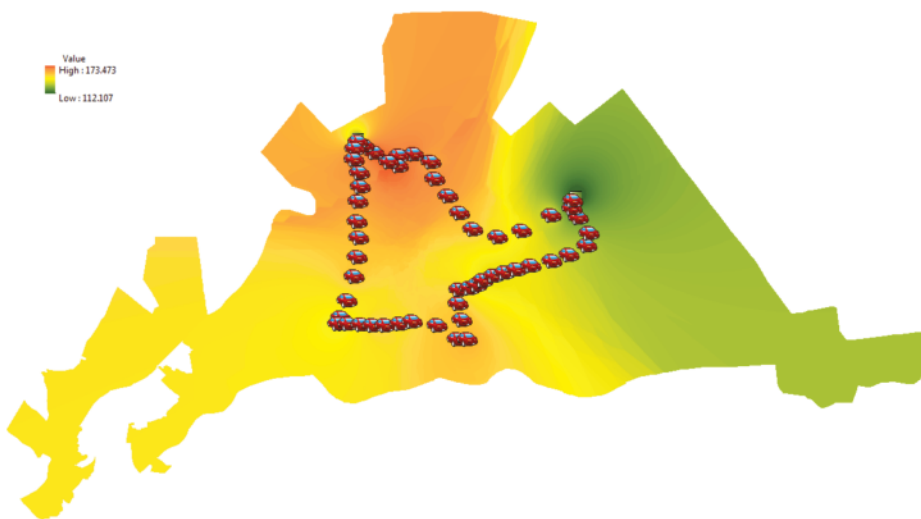
Figure 7. Air quality map provided by the mobile sensor traversing the city. When the sensor travels the path shown in Figure 6, the air quality index gradually changes and this new information becomes updated for the streets of the city.
